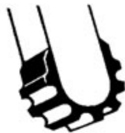
EXTENSION SHOE Reinforced neoprene. Ladder rail must be shaped to fit. Furnished in pairs. 1" and 1-1/4" width. Specify width when ordering.
